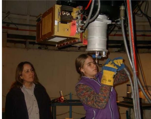
**Figure 2:** Marsha Wolf (l) and Susan Hollis (r) filling the dewar with LN<sub>2</sub>. Credit: S. Sims
